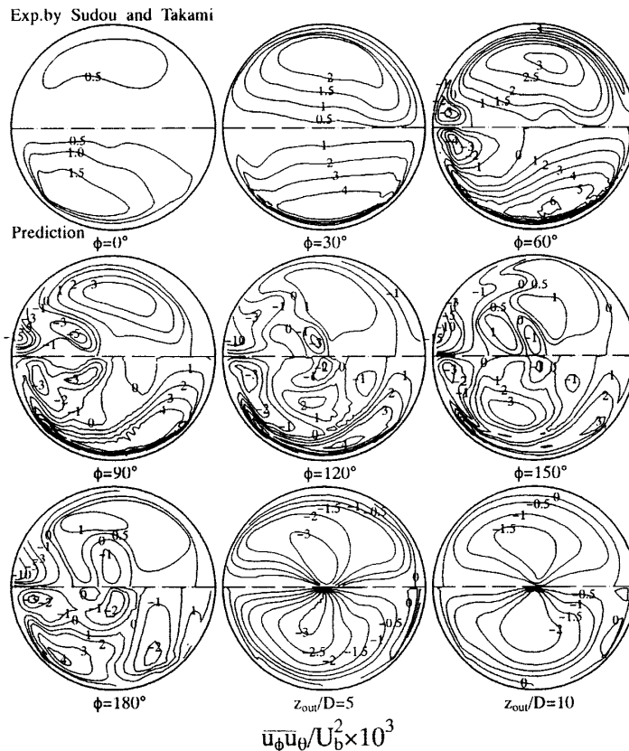
Fig. 9 Comparison of shear stress \overline{u_\phi u_\theta}
